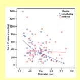
The lines of best fit suggested that the burst strength was more consistent across the diameter range with the LOTUS, while there was a steady decline in burst strength as vessel calibre increases with the Harmonic Scalpel. For vessels of diameter above 5.2 mm, this difference became significant.
