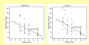
Higher temperature rise with the LOTUS at distances 2 to 4 mm from the cut edge. Thermal spread was insignificant at distances above 5mm with both devices.
