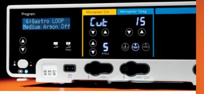
GastroCut offers protection against perforation with polypectomies, papillotomies or endoscopic resections with loops or needle electrodes
