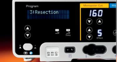
The resection program allows for the use of 300 W for vaporisation with monopolar resectoscopes
